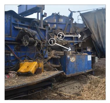
Worker stood on fuel tank (1) to remove jam from chipper (2) when he fell less than 5' and broke his neck.
