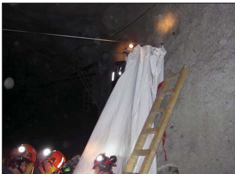
The barricade hangs like a shower curtain and is easy to open.
