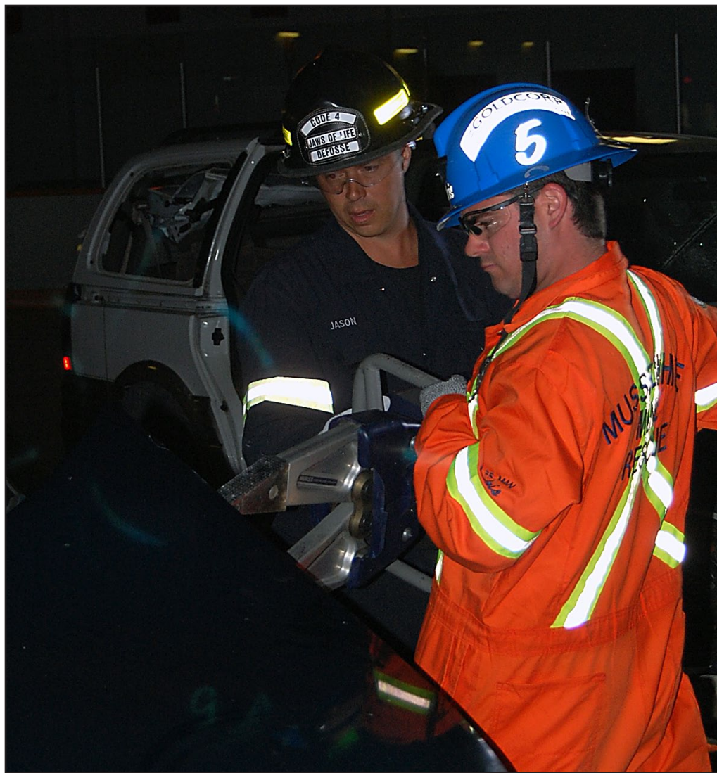
Open wide! A trainer guides a mine rescue volunteer using a Hurst eDraulic Spreader during a demonstration exercise at the 2013 Provincial Mine Rescue Competition.
