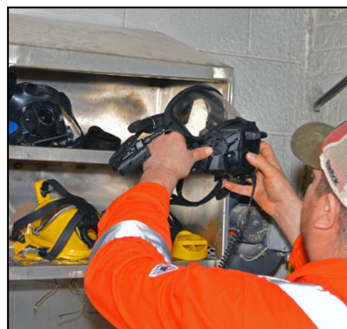
The facemask and communication module can be immersed in water, above, and heat dried, below.
