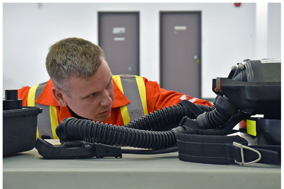
TOP TECHNICIAN - Vale Canada's Jean-Yves Doiron gets upclose to a BG4 requiring servicing during the Ontario Mine Rescue Provincial Competition.
