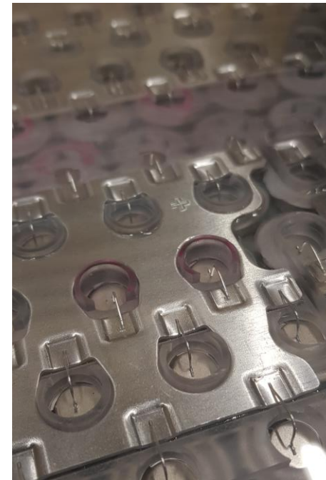
Cells connected via wirebonds
