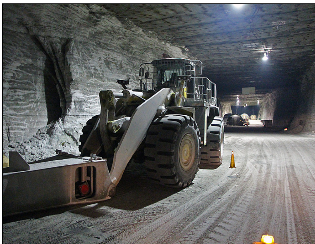
SAFE TO CROSS – A drift in Compass Minerals Goderich Mine is more than wide enough for two-way heavy equipment traffic.
