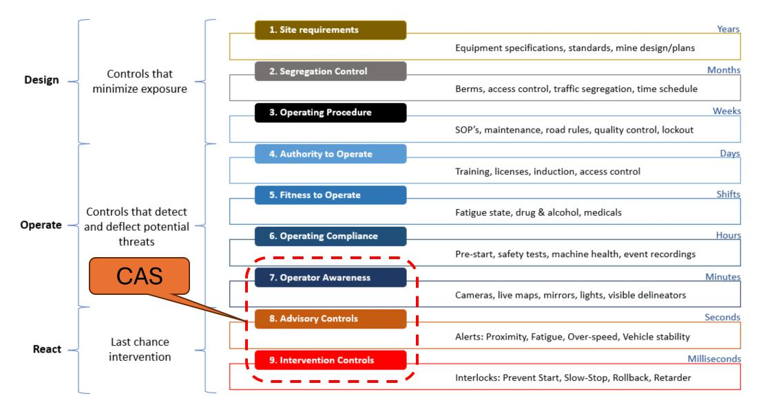
The EMESRT Nine Layer Model for Improving Vehicle Interaction Controls
