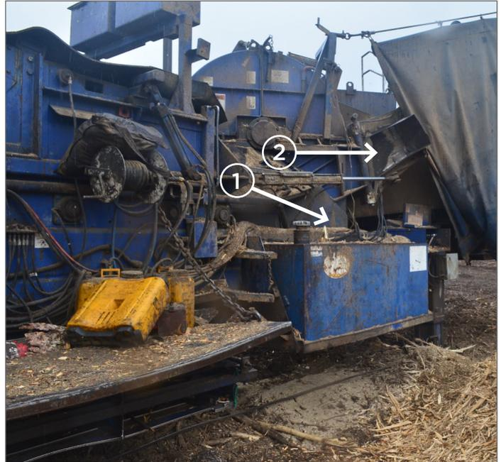
Worker stood on fuel tank (1) to remove jam from chipper (2) when he fell less than 5' and broke his neck.
