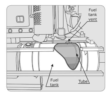
In this fuel tank vent system, the vent allows excess pressure and vacuum buildup in the tank to escape through a narrow tube (shown above on the far side of the tank) that discharges near the ground.
