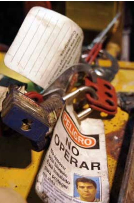
Lock out, tag out: systematic locking out and tagging out keeps maintenance safe.
