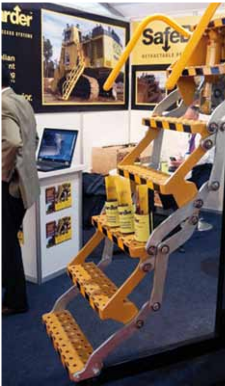
Safety played a huge role at Exponor Antofagasta: on display here is a safe access system for earth-moving machines.
