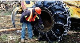
thorough circle check should be an automatic step to using a vehicle or mobile equipment for the first time each day, and is an important step in ensuring a safe workplace.
