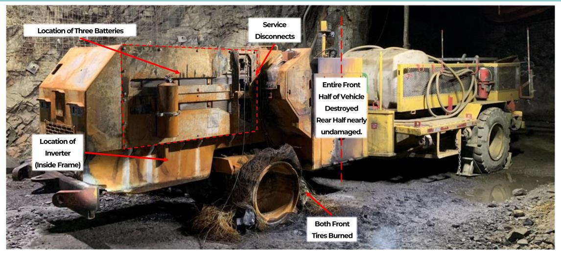
Figure 2 – Post-Incident Photo of BEV
