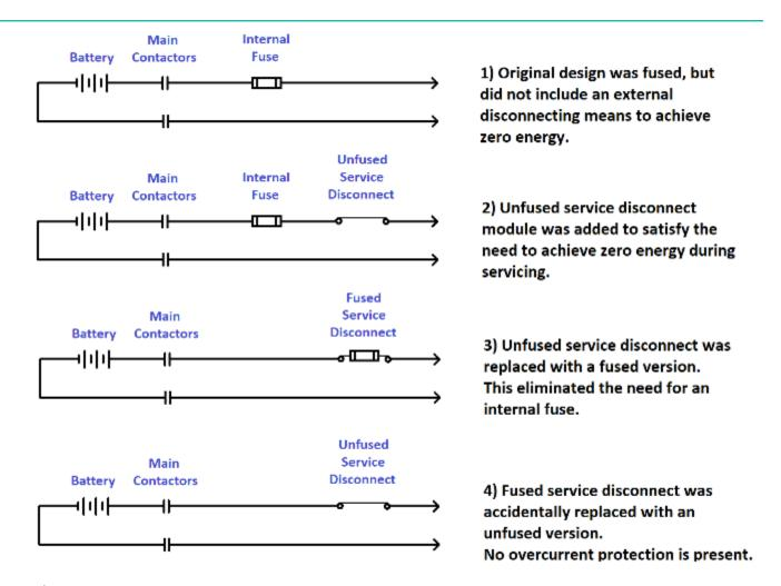
Figure 11 – Simplified Schematics depicting modifications to fuse arrangement.
