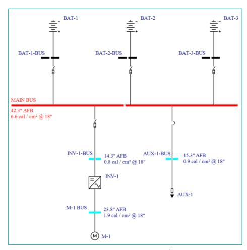
Figure 14 – Example of Electrical Single Line / Model
