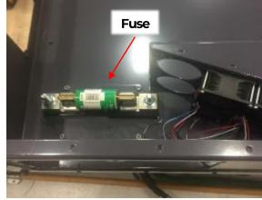
Figure 3 – Original Battery Fuse
