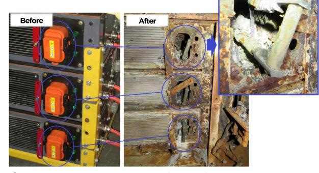
Figure 9 – Manual Service Disconnects – Before and After Incident
