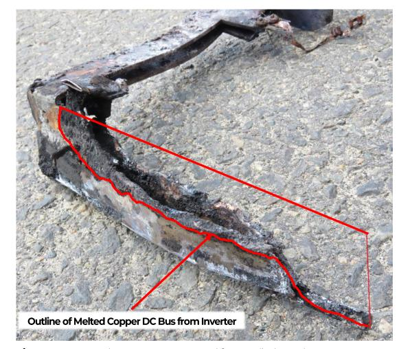
Figure 10 – Internal DC Bus Bar extracted from Failed Traction Inverter
