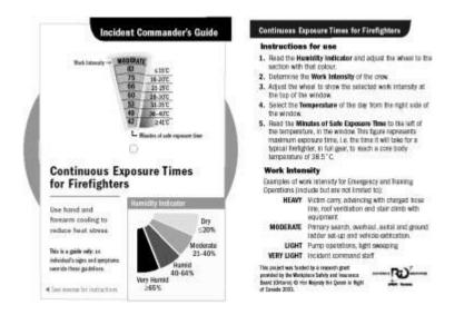
Controls recommended by the research include, if possible, varying the workload intensity by rotating or alternating responsibilities, withdrawal from the heat zone to permit on-site recovery and cooling, immediate access to water for rehydration, removal of personal protective equipment and clothing, as well as the active cooling methods of hand and forearm submersion in water, and cooling mists.
