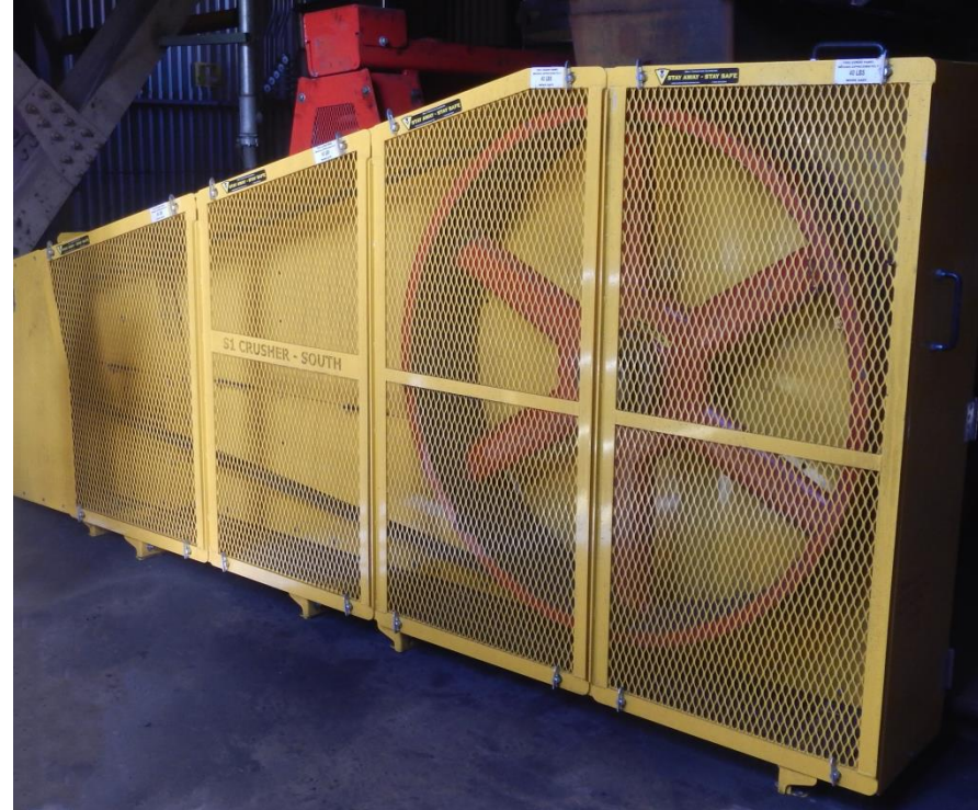
Example of guarding the flywheel of a crusher. (source: Belt Conveyor Guarding).
