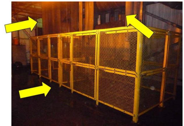
Two conveyor gravity take-up counterweight guarding (source: Belt Conveyor Guarding)
