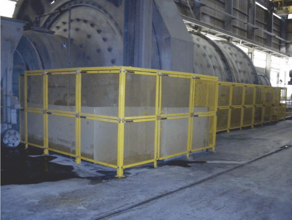
Example guarding in the vicinity of a grinding mill (source: Belt Conveyor Guarding).
