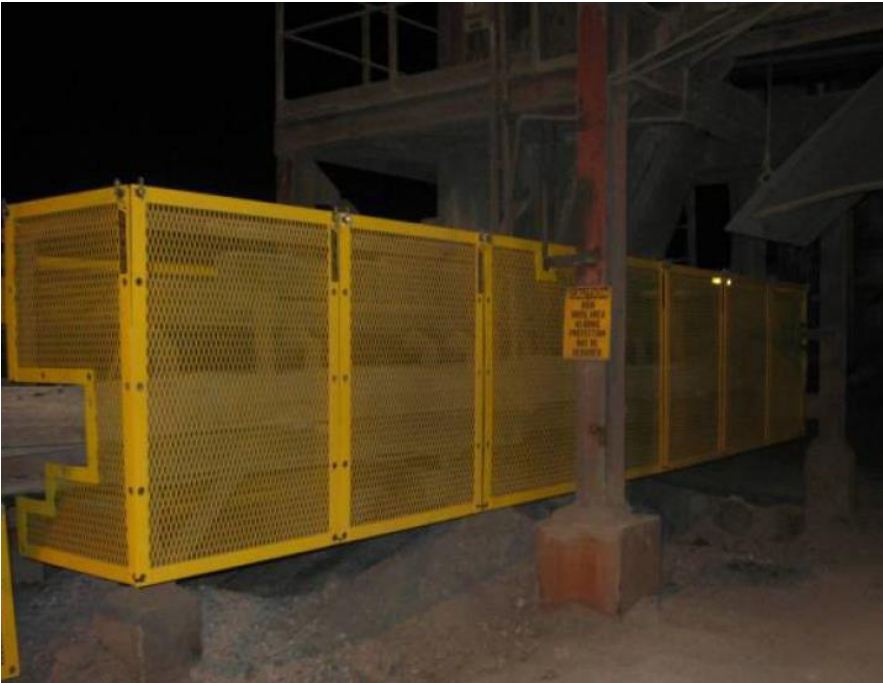
Example guarding in the vicinity of a hopper (source: Belt Conveyor Guarding).
