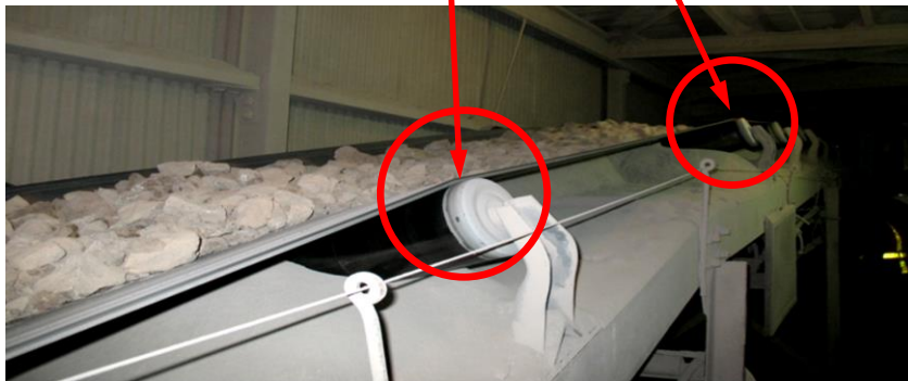
Unguarded pinch point - convex curve of a belt where the lift is restricted must be guarded (Section 196.(3)(2.)).
