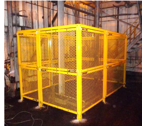
Single conveyor gravity take-up counterweight guarding (source: Belt Conveyor Guarding)
