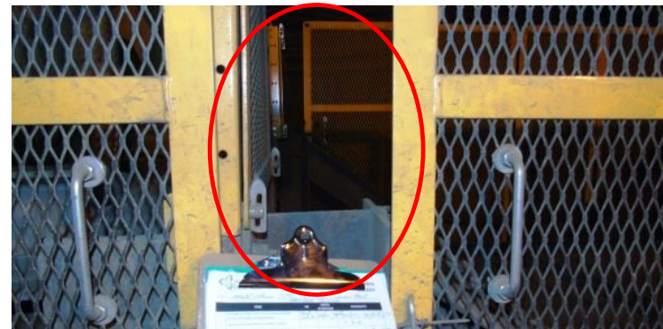
Guarding example with excessive space between guards are noted where the whole upper limb or extremity of a person can be inserted.
