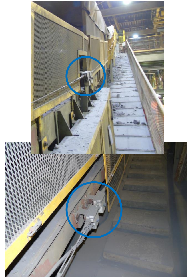
Example of clearly visible and properly installed pull cord and re-set button.
