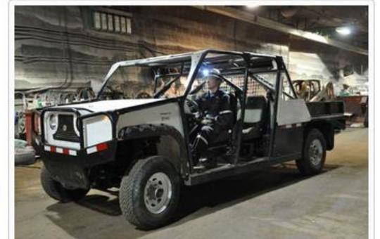
Thanks to NRC-IRAP support, Saskatoon's PapaBravo Innovations developed a line of rechargeable electric vehicles for the mining sector to replace the diesel-guzzling trucks currently in use – eliminating noxious fumes in the process.
