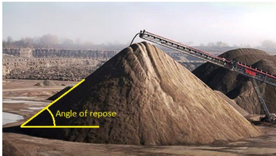
Figure 1 - Stockpile angle of repose
