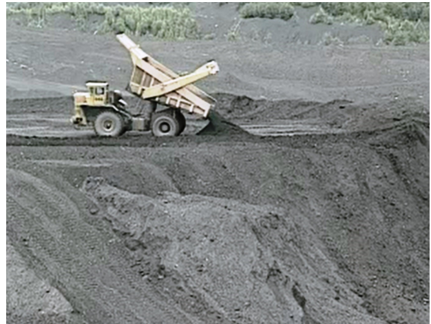
Figure 5 - Haul truck dumping back from the crest (source: MSHA Stockpile Video,
