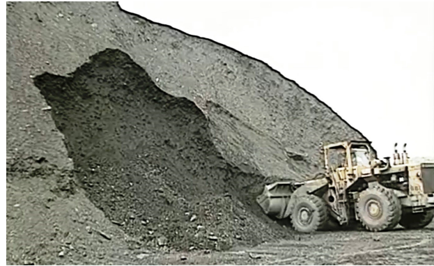
Figure 4 - Undercutting of stockpile
