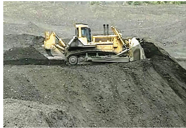
Figure 6 - Dozer pushing over the edge (source: MSHA Stockpile Video, 1994)
