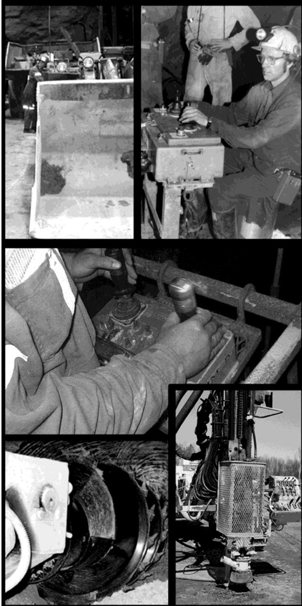
Early units used radio controllers transmitting coded messages on a carrier frequency. The radio frequencies of the sending and receiving units had to match. The receivers connected with a machine's electric, hydraulic and pneumatic systems to control functions such as steering, braking and load handling.
