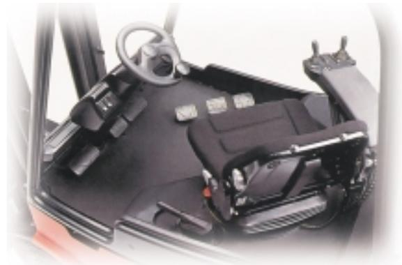
*B -- a swivel seat, and dual pedals are a good start to designing a better lift truck.*
