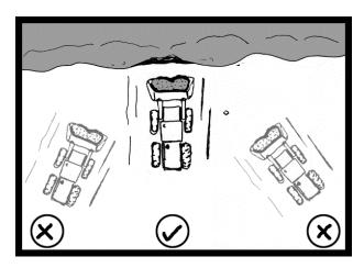
at the angle of repose or the vertical height of the working face shall not be more than 1.5 metres above the maximum reach of the equipment.
