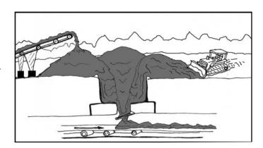
Mobile equipment shall not be operated directly over a draw hole.
