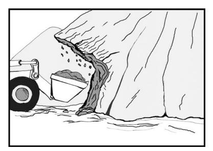
Excavations shall not undercut or leave a concave hollow in the material. Operators will not cut trenches or tunnels into the slope or leave any overhangs in frozen material.
