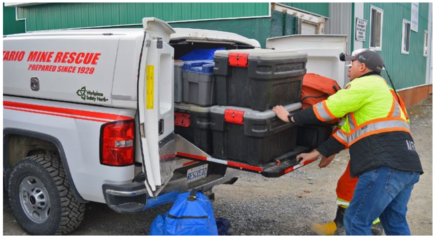
OMR transitioned from cargo vans to 4WD pickups for improved handling, and to better deal with accumulated mileage, poor weather, rough road conditions and terrain - 2015
